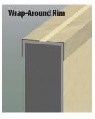
Wrap-around rims may not require flashing or caps to be fully functional.
